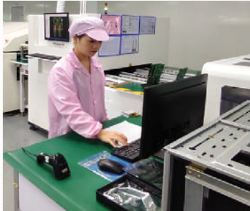
AOI check For: Reflux welding PCBA, component welding conditions for automated testing.
