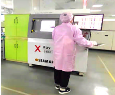
X-Ray check For: BGA/QFN type component solder inspection.
