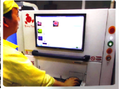
SPI check For: Full automatic solder paste printing effect inspection.
